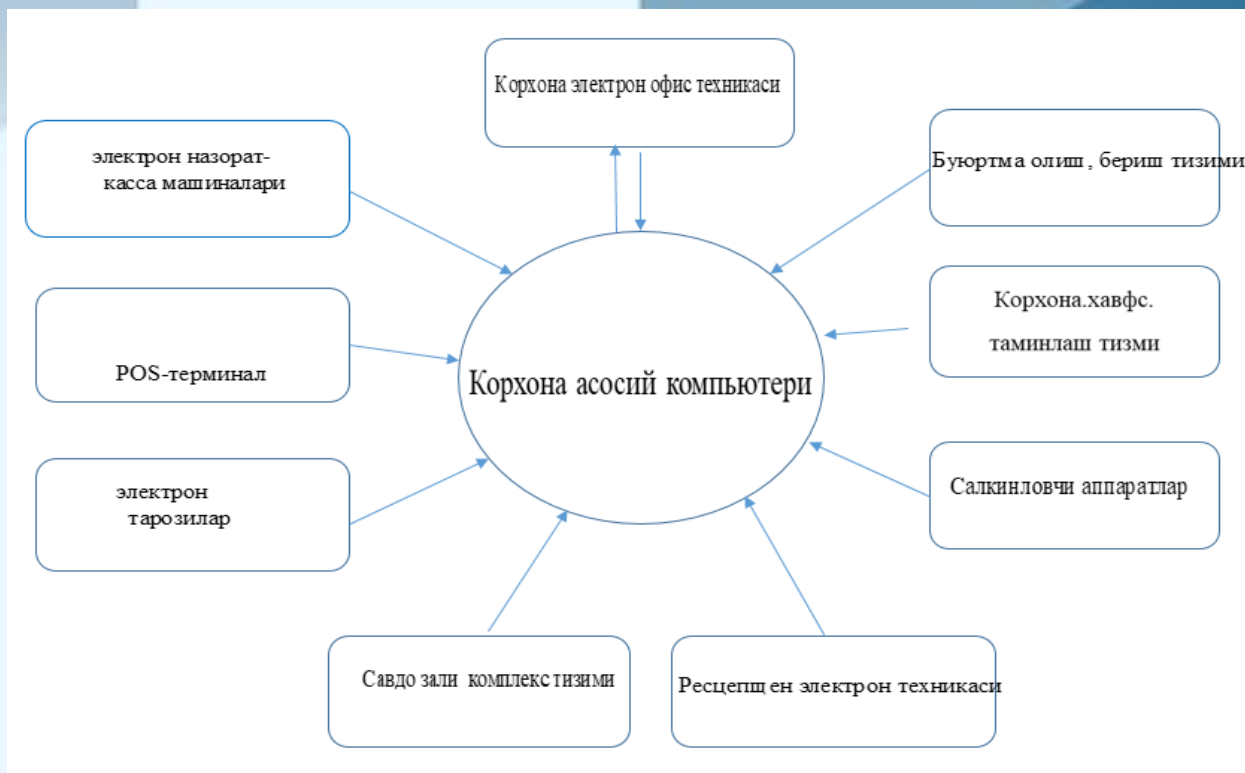
Figure. 1. Samarkand sh. The principle scheme of the topology of the restaurant "Amir" and the network system "Korzinka" supermarket in the form of "Star".
